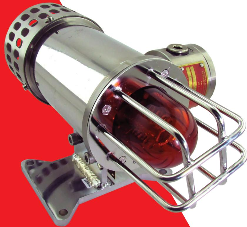
This electronic sounder and LED beacon combination unit is suitable for use in fiery mines as well as petrochemical plants and areas where an explosion-protected device is required. The unit consists of a 304 type stainless steel housing with a M20 cable entry, a stainless steel nose cone and a unique screw on lid for cable connection.
