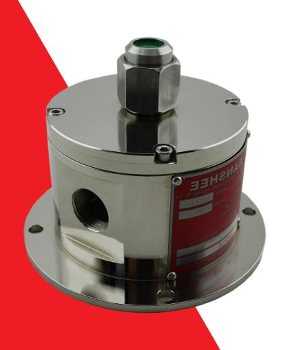
The Banshee Ex Start Station S3 enables operators to safely initiate the operation of machinery and equipment used in underground mining applications. The unit consists of a flameproof enclosure that houses a switch operator which supplies power to the equipment when the start button is pressed.
